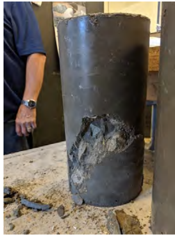
Broken concrete cylinder from materials testing activities, - USAF Camp, Scott AFB -
